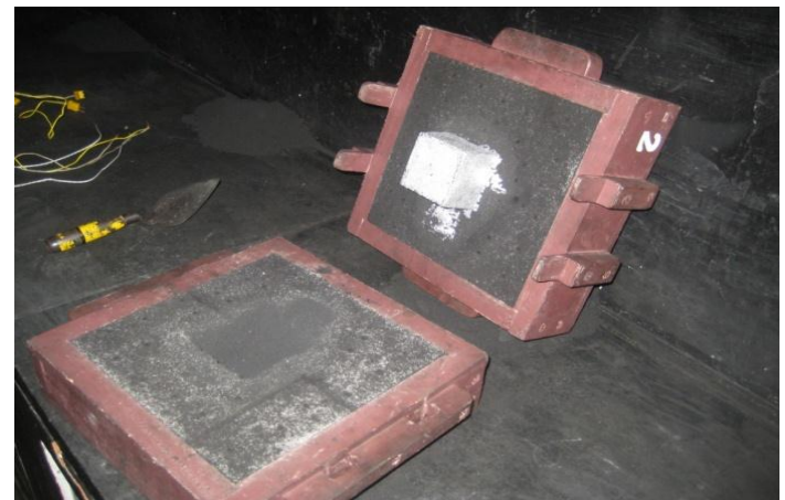
Figure 2 Sand packed into a flask in conventional method.
